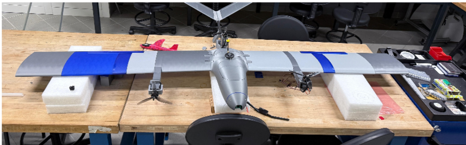
3.4 kg team-built prototype during integration and testing
